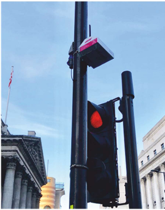
Graphic 2.2 Example of a real-time particulate monitor
