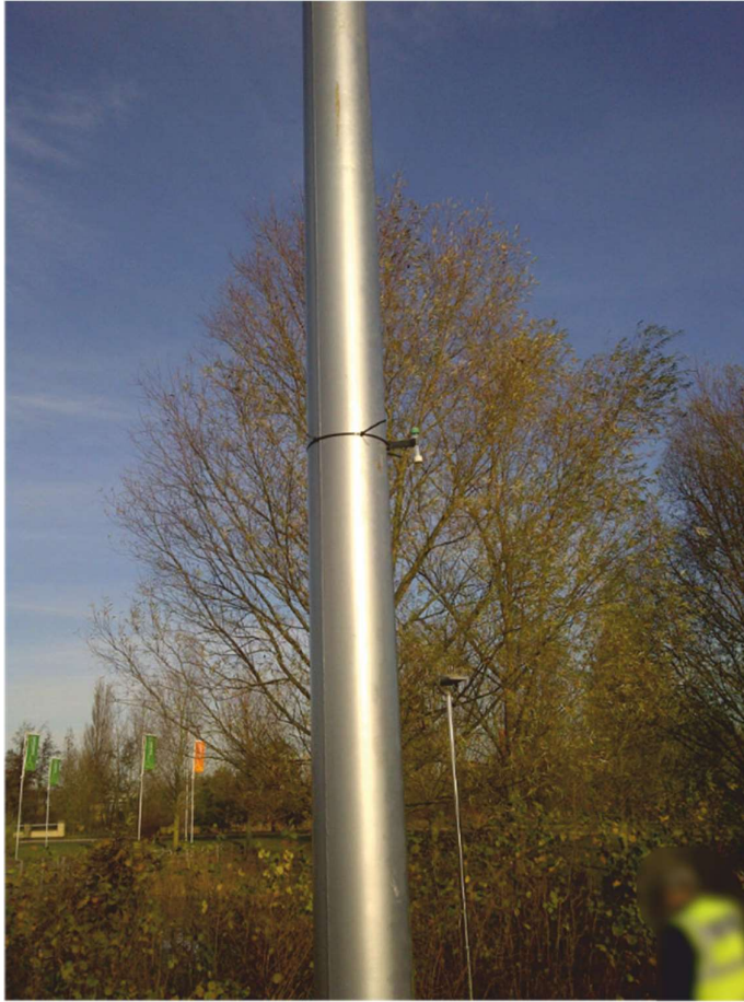
Graphic 2.23 Example of a passive air quality monitoring diffusion tube
